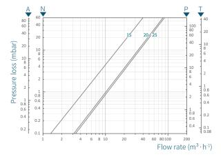
A: Air 1.2 kg⋅m<sup>-3</sup>, N: Natural gas 0.75 kg·m<sup>-3</sup>, P: LPG 2.0 kg·m<sup>-3</sup>, T: Town gas  $0.55 \text{ kg} \cdot \text{m}^{-3}$ . Gas temperature: 20°C.
