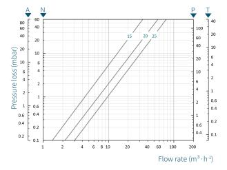
A: Air 1.2 kg·m<sup>-3</sup>, N: Natural gas  $0.75 \text{ kg} \cdot \text{m}^3$ , 2.0 kg·m<sup>-3</sup>, P: LPG T: Town gas  $0.55 \text{ kg} \cdot \text{m}^{-3}$ . Gas temperature: 20°C.
