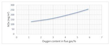
For different air excess coefficient NOx (ref. 8% O<sub>2</sub>).
