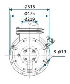
Pilot burner gas access Rp1/4", air access Rp1/2".
