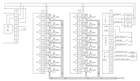
There are four rows of terminals: X1, X2, X3 and X10 on the back of SPC 108. X1 are the terminals for input signal and output signal; X2 are the terminals for output channel 1~4; X3 are the terminals for output channel 5~8; and X10 are the terminals for the input and output of power supply.
