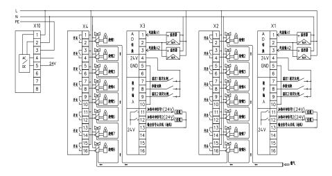
There are four rows of terminals: X1, X2, X3, X4 and X10 on the back of SPC 216. X1 are the first set of terminals for input signal and output signal; X2 are the terminals for output channel 1~8 corresponding to the first set of input signal; X3 are the second set of terminals for input signal and output signal; X4 are the terminals for output channel  $1\sim$ 8 corresponding to the second set of input signal; and X10 are the terminals for the input and output of power supply.
